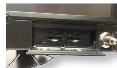
Tamperproof lockable MicroSD Card Compartment
