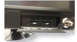
Tamperproof lockable MicroSD Card Compartment
